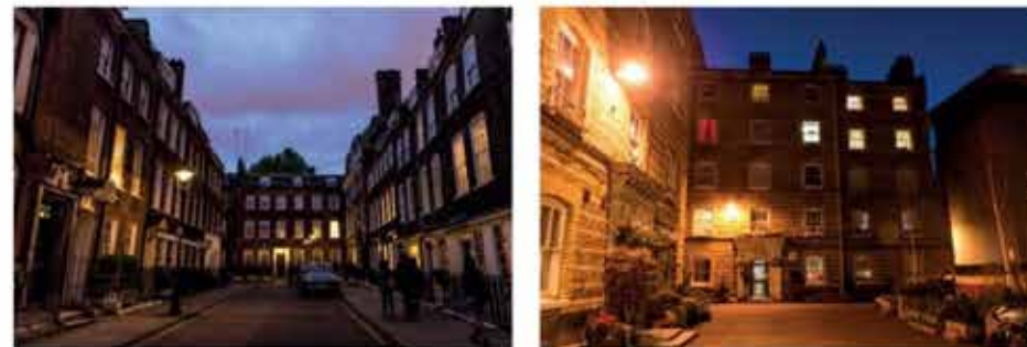
Figure 1. These two images show the lighting for (left) a residential street in central London versus that within a social housing estate. This illustrates how lighting levels, installation height, colour of light and the appearance of fixtures creates an astonishingly different environment. Photograph by Caterina Heckl
